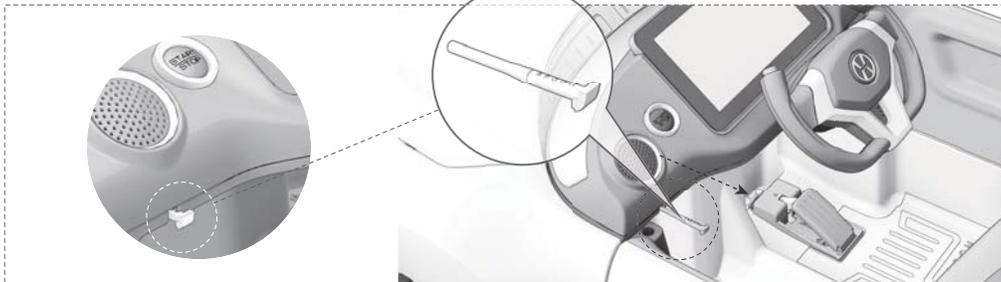
※ In order to open the bonnet, the opening key located below the dashboard need to be separated.
