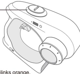
※When in emergency stop mode, the LED indicator blinks orange.
