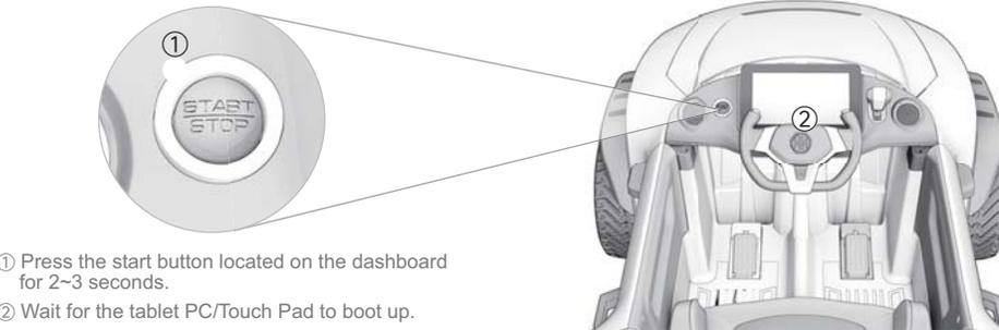
※After use, the vehicle must be turned off by using the start button.
